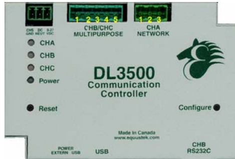
Pin Numbering for the DL3500
