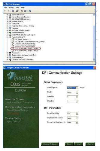
Find out what COM port has been assigned to the DLPCIE. To do this, open the Device Manager (from the Control Panel, select System, then on the Hardware tab in the System Properties window, select Device Manager). Under *Ports* (*COM & LPT*) you will see the two COM ports assigned to the DLPCIE Use the 1<sup>st</sup> one, as the second one is the DB9 pin RS232 general purpose serial COM PORT.
