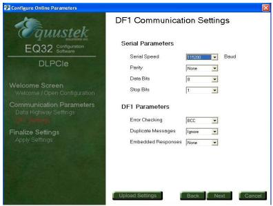
Click on Next and make sure that the unit is in configure mode other wise press the configure button as shown below.
