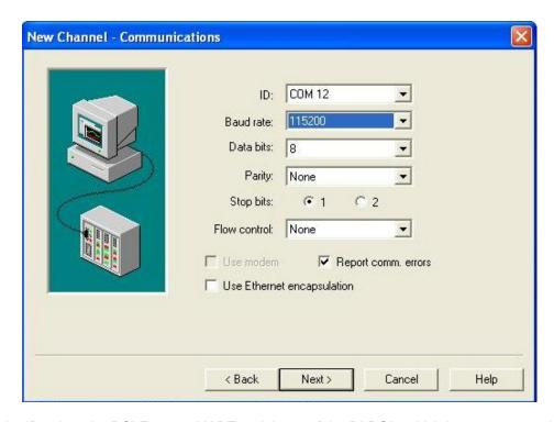
Under ID select the PCI Express UART serial port of the DLPCIe which in our case as shown in the 1<sup>st</sup> screen shot is COM12.
