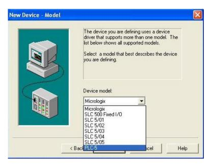
Here you select the device ID (It is the DH+ node address number of the Processor ) in my case my PLC5 node address number is 7 and make sure to match it in either Decimal, Octal or Hexadecimal. AB devices usually use the Octal
