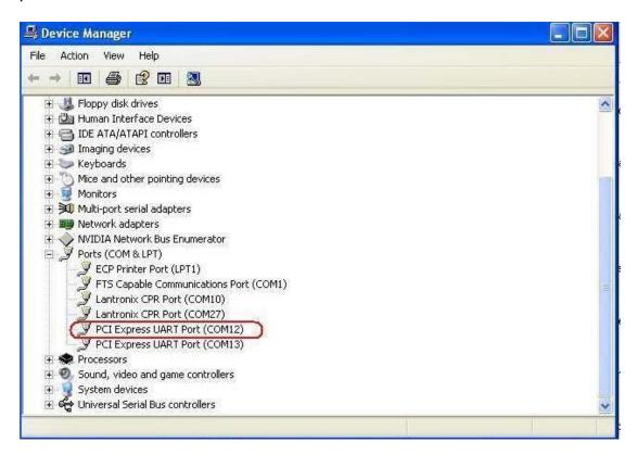
COM13 is a general purpose serial port can be used as any RS232 serial port.
