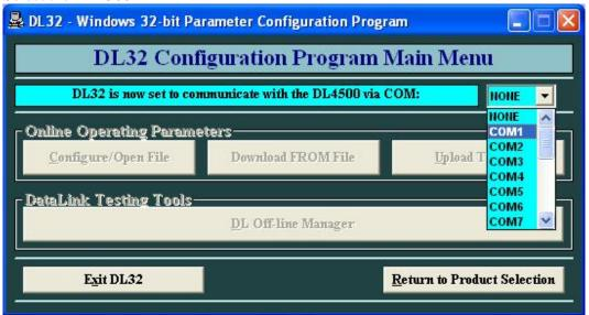
Select the serial port that is connected to the DL4500 DB9 connector. And then click on DL OFFLINE Manager
