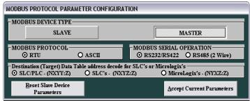
*Example 1:* B18:30 (xy:z) will access register 00030 from Modbus Slave address 18.
