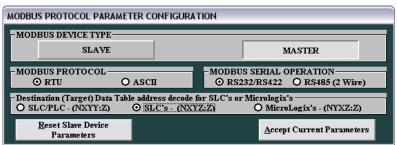
Use this format if the ControlLogix or other devices allows up to 999:999 to be entered for the file and word. The file goes up to 999 and the word up to 999. *For this format, your register address should be between (1 to 9999)*.
