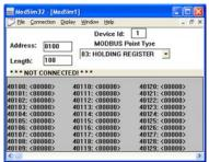
Device Id is the Modbus Slave ID, Address is the Register address, Length is the number of registers, Modbus Point Type is 03 Holding Registers.
