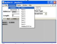
From the drop menus select the serial settings similar to the unit configuration and the Modbus device.
