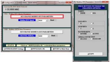
Click on SET/CHANGE MODBUS ASCII PARAMETERS, and select the settings similar to those that match your MODBUS ASCII device.
