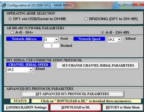
Press the Configure Push Button Switch on right hand side of the DL3500 then click on OK.
