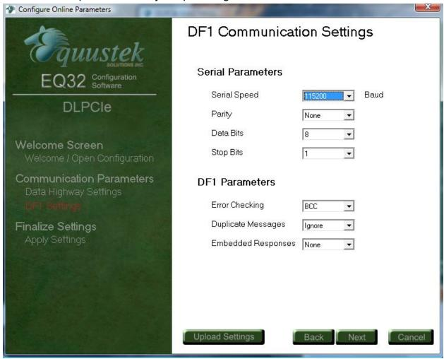
If different settings are required please use the EQ32 to configure the unit with the EEPROM as shown in the previous step.
