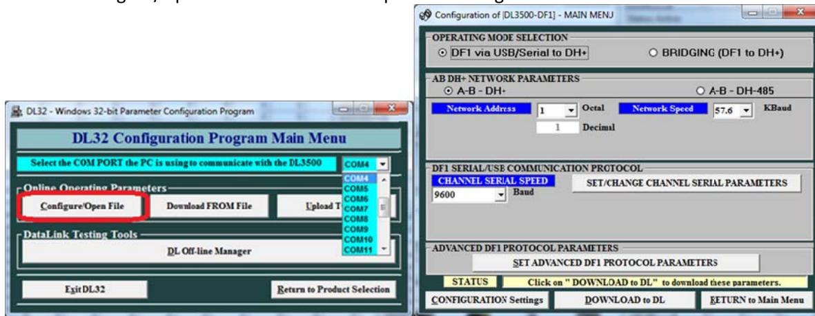
Check the serial settings for the DF1 channel of the Micrologix to make sure they match the settings for the DF1 channel of the DL3500. For DL3500 Operating Mode Selection, select DF1 via serial to DH+, then select the DH+ node address, DH+ baud rate
