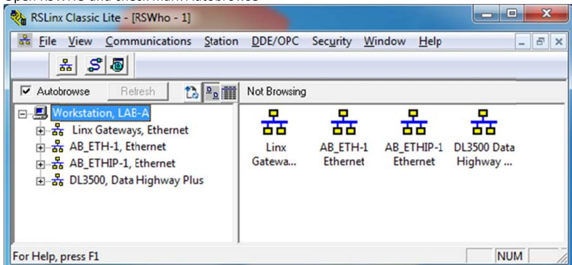
When you Click on the RS232 DF1 driver that was created (DL3500), you should see all the PLCs that are on DATA Highway plus Network as shown below.
