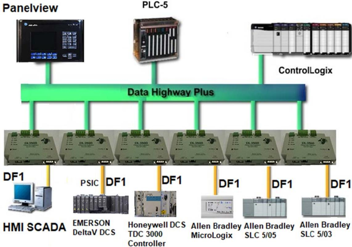
**DL3500-DF1/DH+ allowing DF1 Devices to Communicate with DATA HIGHWAY PLUS PLCs & Devices**
