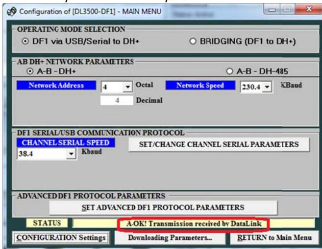
Once setting are downloaded press the RESET push button switch on the left hand side of the DL3500 and click on OK here.
