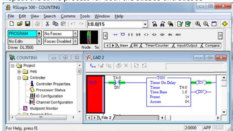
If you have a Honeywell DCS TDC 3000 or Emerson Delta V DCS same will apply when the serial DF1 settings of DL3500 are configured with matching DF1 settings of the TDC3000 or DELTA-V then the DH+ PLCs will see the DCS like any other DH+ device and will be able to communicate with each other similar like any other Data Highway Plus Device.
