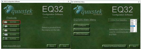
From the drop Menu of the COM Port Selection, select the USB comport previously found under the Device Manager.
