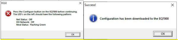
In case you encounter any error message, press the **RESET push button switch** on left hand side of the EQ7000 then press the **Configure push button switch** on the right hand side of EQ7000 and click on Finish again in EQ32.
