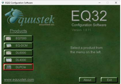
Once the DLPCIe card is installed in any desktop PC it will occupy 2 serial ports one of them is just an extra serial port for the PC while the other one is the serial port that will be used for the serial communications with the card using Allen Bradley serial RS232 DF1 protocol, both those ports can be found under Ports(COM&LPT) in Device manager.
